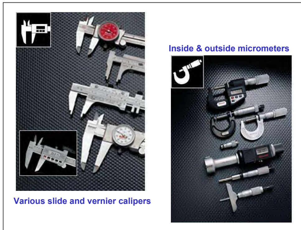
Figure 3-8. Assortment of Starrett micrometers and calipers that can be used for measuring short distances in concrete structures to an accuracy of 0.0005 inch or better.
